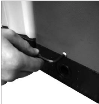
2. Remove single retaining screw.
