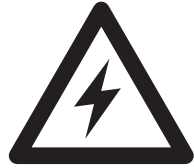
Caution: Risk of Electric Shock
