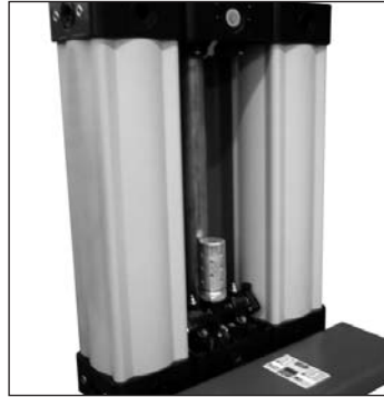
4. Dryer with front facia panel removed.
